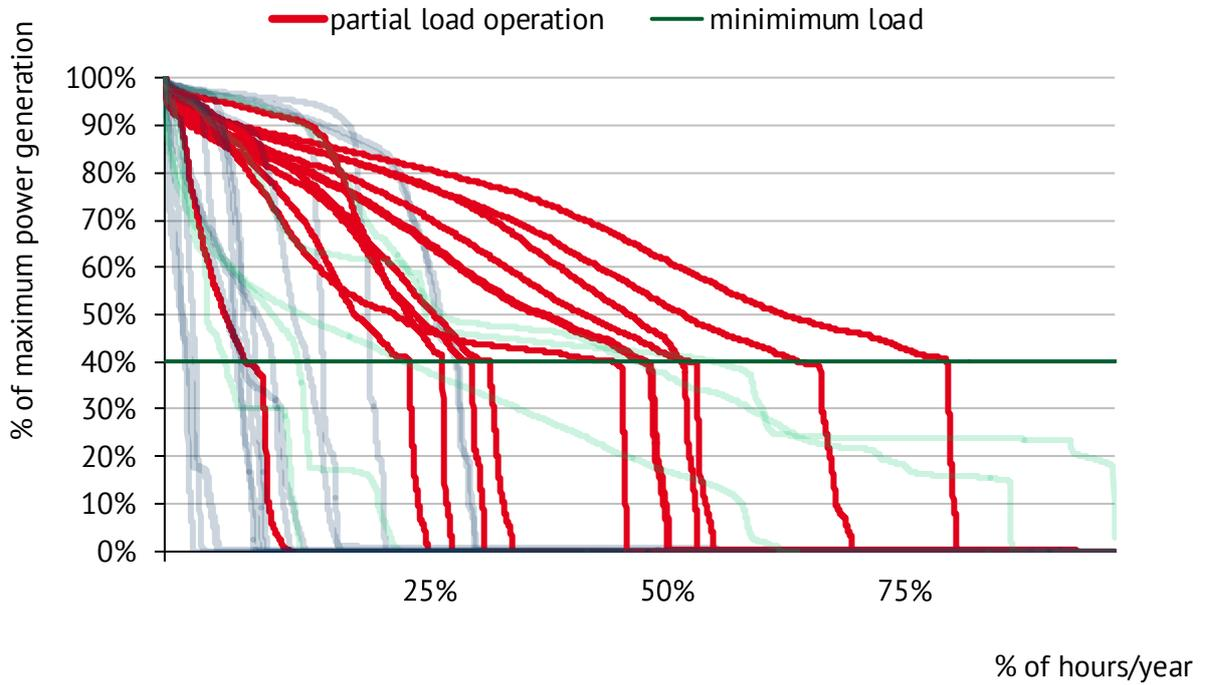
Figure 14: Sorted annual load curves of 12 gas-fired power plants in the “partial load operation mode” in France, Germany and Spain (Source: EEX, Entsoe)
