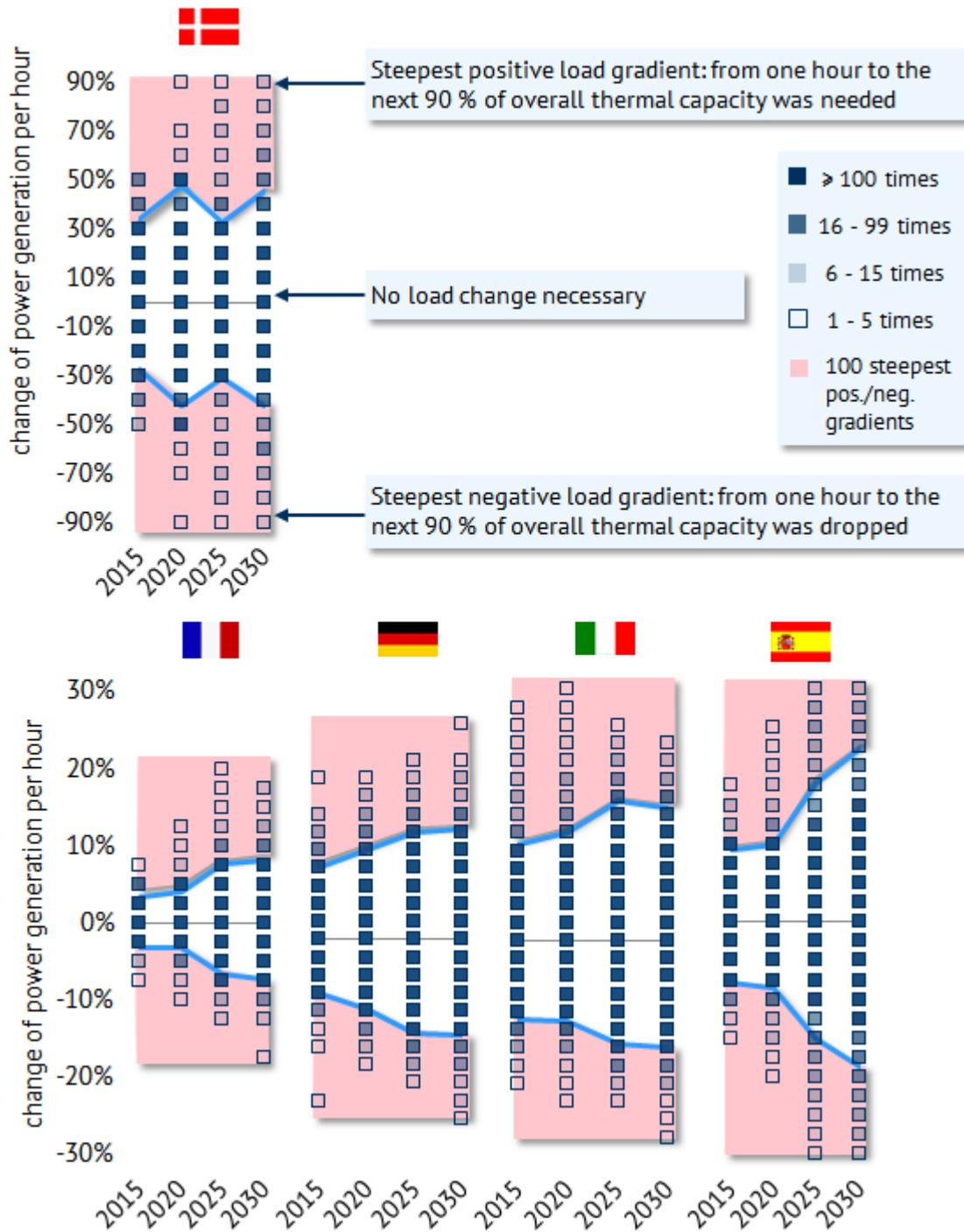
Figure 11: Development of the change in use of thermal power generation in different countries in % of maximum power generation per year
