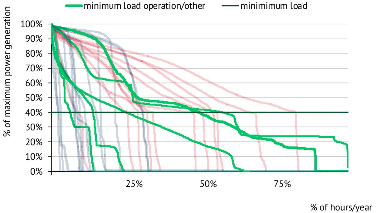
Figure 16: Sorted annual load curves of 9 gas-fired power plants in the “minimum load operation mode/other modes” in France, Germany and Spain (Source: EEX, Entsoe)
