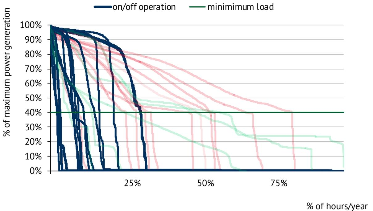
Figure 15: Sorted annual load curves of 11 gas-fired power plants in the “on/off operation mode” in France, Germany and Spain (Source: EEX, Entsoe)
