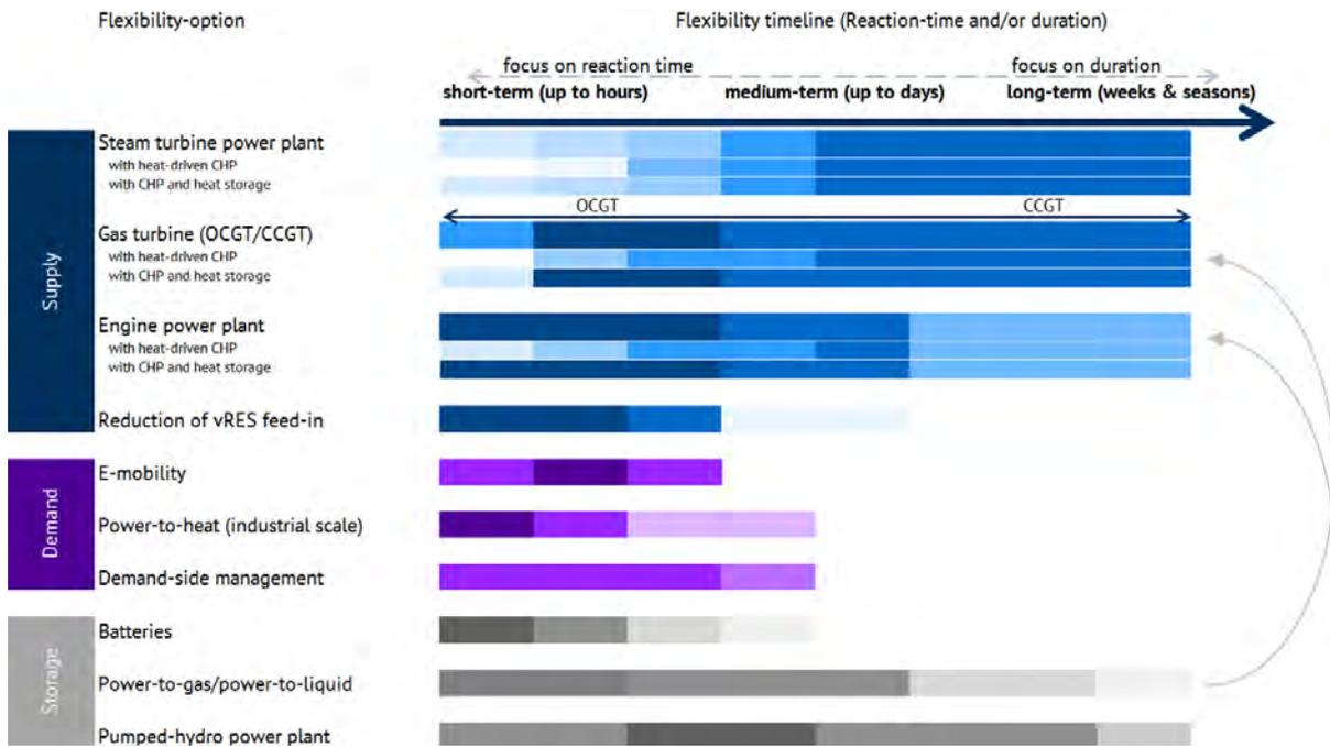
Figure 4: Flexibility options along the flexibility timeline (CHP: Combined Heat and Power, OCGT/CCGT: Open/Combined Cycle Gas Turbine, vRES: variable Renewable Energy Sources)
