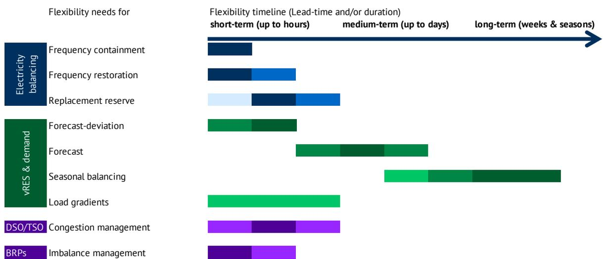
Figure 2: Flexibility needs along the flexibility timeline (vRES: variable Renewable Energy Sources, DSO: Distribution System Operator, TSO: Transmission System Operator, BRP: Balancing Responsible Parties), lead time is more important for short-term flexibility, duration is more important for long-term flexibility
