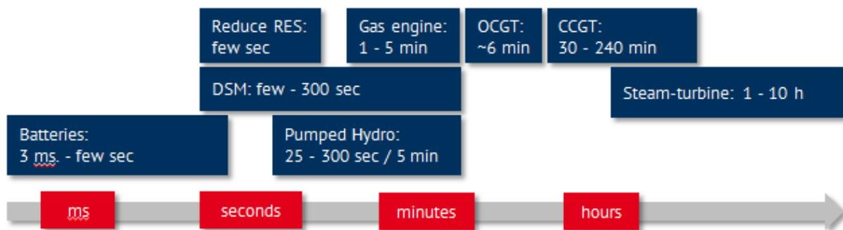
Figure 7: Reaction time from command to full load of selected flexibility options
