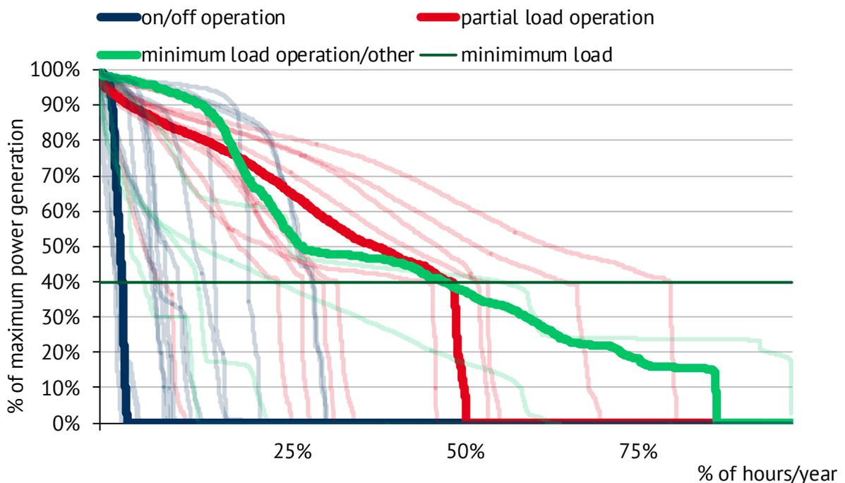
Figure 8: Sorted annual load curves of three characteristic operation modes and of in total 30 gas-fired power plants in France, Germany and Spain (Source: EEX, Entsoe)
