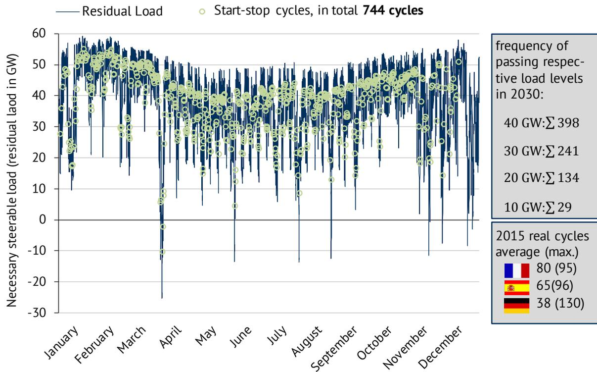
Figure 12: Hourly necessary steerable load in 2030 and start-stop cycles in comparison to real cycles in 2015
