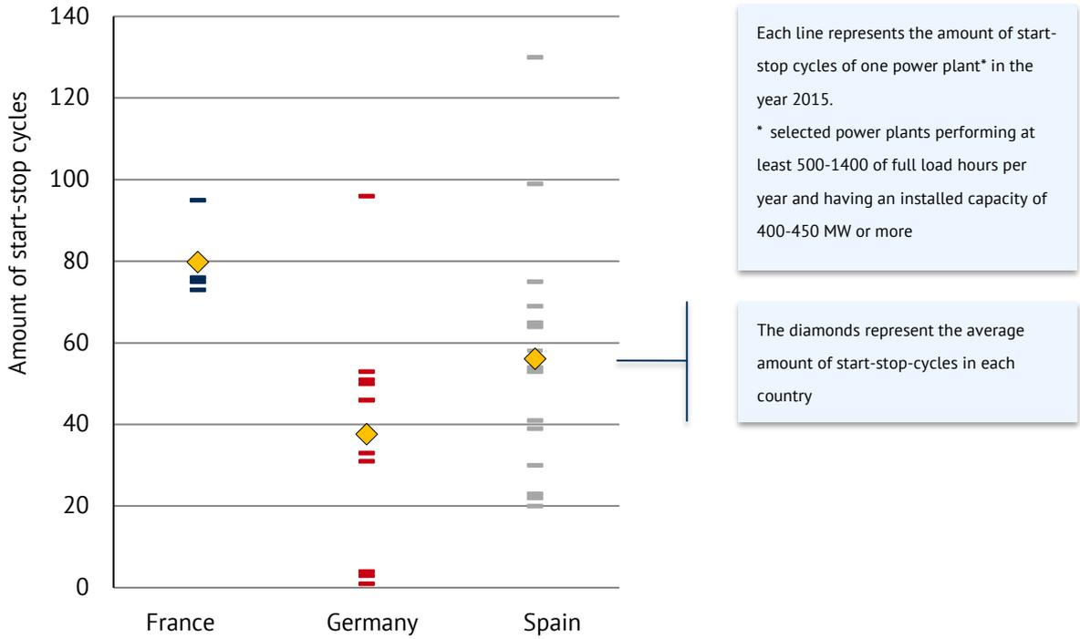
Figure 17: Amount and average of start-stop cycles of gas-fired power plants per year in different countries (source: EEX, Entsoe)
