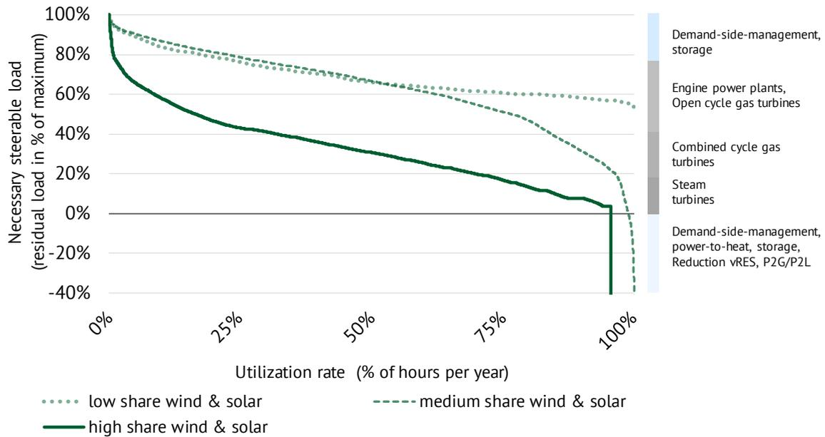
Figure 5: Exemplary analyses of potentials for flexibility options following the sorted hourly residual load curves of power systems with a high (solid), medium (dashed) and low (dotted) share of wind & solar.
