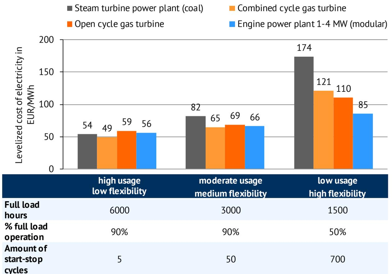
Figure 9: Levelized cost of electricity depending on character of operation (usage/flexibility), Different use cases for the operation of power plants, high usage with low flexibility (coal power plants today), moderate usage with medium flexibility (gas-fired power plants today) and low usage with high flexibility (use case for flexible power generation in the future)
